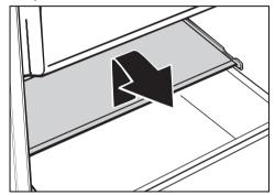
Lift the front edge of the plate out of its holder and pull the plate out of the appliance.
